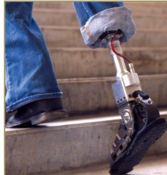
VA has supported the development of a powered ankle-foot prosthesis that will help patients walk faster with fewer balance problems, and a neurally controlled arm and hand prosthesis that will perform, look, and feel like a natural limb, making handling objects much easier.
