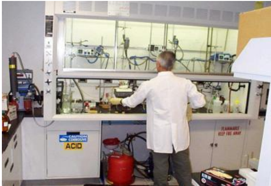
Figure 6-4: Fume Hood with a Vertical Sash at Restricted Height Design Opening (Source: Lawrence Berkeley National Laboratory , 2006)
