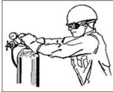
Figure 8-9: Proper Position for Opening a Regulator (Source: Virginia Tech Environmental Health and Safety , 2011)
