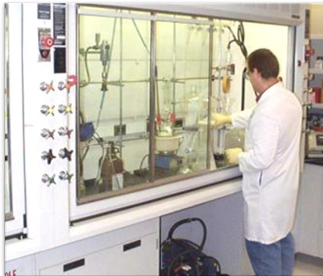
Figure 6-5: Fume Hood with Horizontal Sash Opening (Source: Lawrence Berkeley National Laboratory , 2006)
