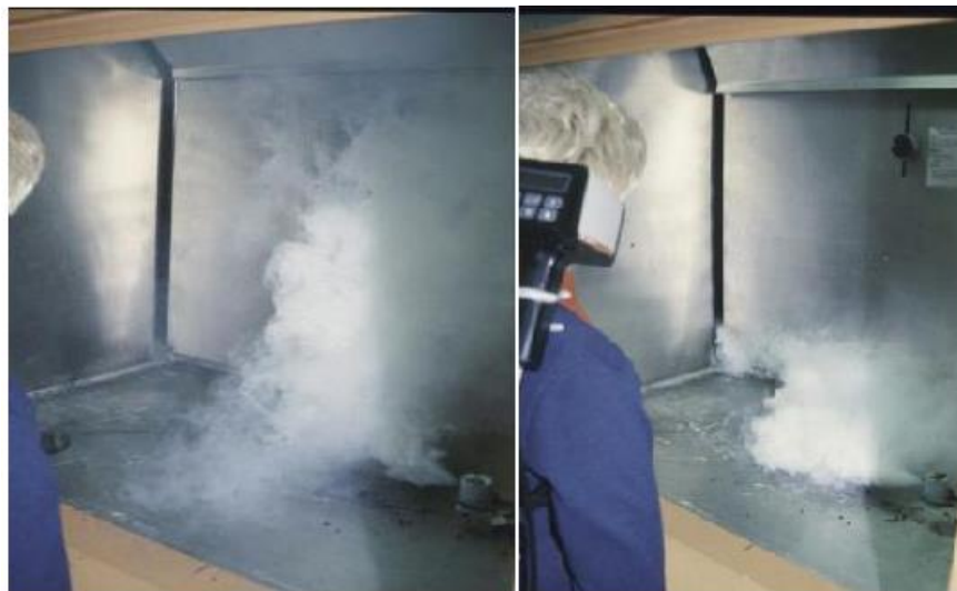
Figure 6-8: Fume Hood Showing Reverse Flow and Escape Near Airfoil Sill with Top Slot Fully Open (Left) and Fume Hood Showing Capture at Bottom Slot with Top Slot Closed (Right)
