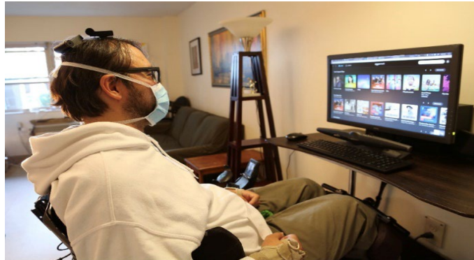
Participant using BrainGate system, with wireless patient cable system (2 black headstages attached to percutaneous connectors), to control cursor on their own personal computer
