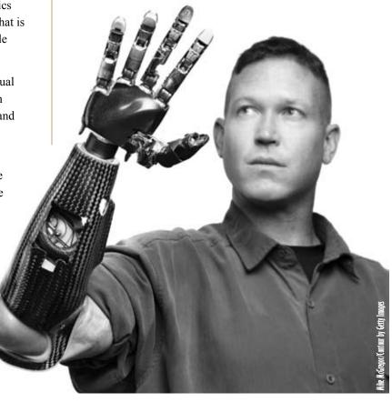
from residual muscles in the forearm. With two electrodes wired to his arm, a senator was able to control the hand and use it to hold a glass of water.
